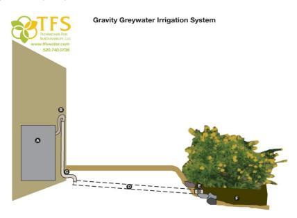
A) Washing machine: Laundry machine can be located outdoors or indoors, near an exterior wall.
